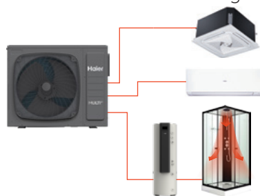
Scenario 2: Domestic Hot Water + AC Heating
