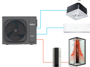
Scenario 5: Domestic Hot Water + AC Cooling
