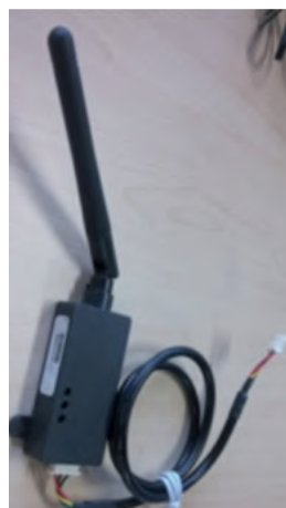
Radio adapter for the indoor unit to be connected to the respective electronic board.
